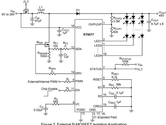
Figure 2. External P-MOSFET Isolation Application
