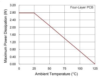
Figure 3. Derating Curve for RT8577 Packages
