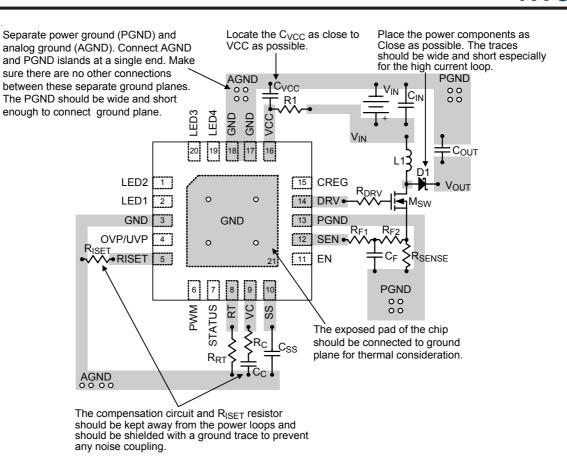
Figure 4. PCB Layout Guide
